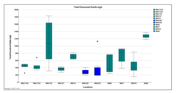
**Figure 3-12.** Box-whisker plot showing distribution of **total dissolved solids** concentration by monitoring well for data collected in 2021 and 2022. Note: Box-whisker plots for background wells are blue and box-whisker plots for compliance wells are green.
