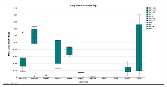
**Figure 3-10.** Box-whisker plot showing distribution of **manganese** concentration by monitoring well for data collected in 2021 and 2022. Note: Box-whisker plots for background wells are blue and box-whisker plots for compliance wells are green.
