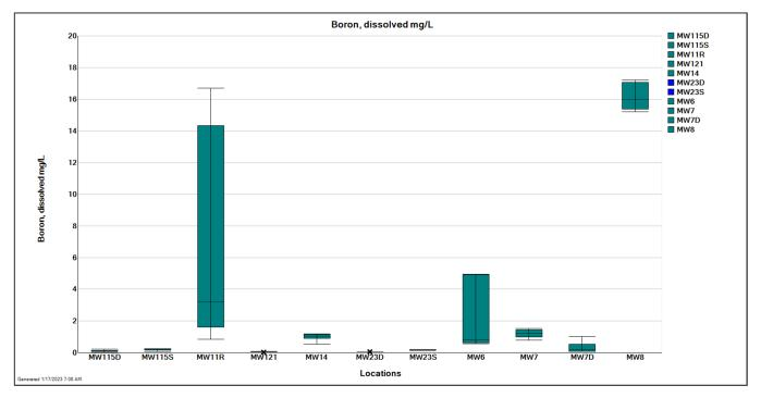
**Figure 3-6.** Box-whisker plot showing distribution of **boron** concentration by monitoring well for data collected in 2021 and 2022. Note: Note: Box-whisker plots for background wells are blue and box-whisker plots for compliance wells are green.
