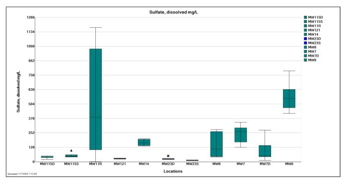
**Figure 3-8.** Box-whisker plot showing distribution of **sulfate** concentration by monitoring well for data collected in 2021 and 2022. Note: Box-whisker plots for background wells are blue and box-whisker plots for compliance wells are green.
