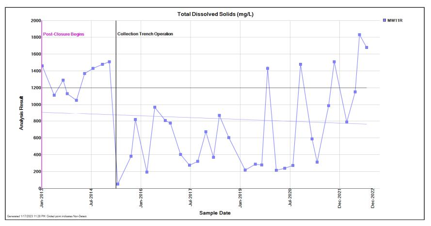
**Figure 4-1.** Total dissolved soilds concentrations over time since closure completion (2013) at compliance wells MW-11R. (Note: Lines through the concentration data represent the best fit linear regressions)
