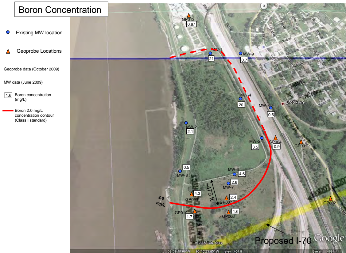
Figure 2. Extent of Class I exceedances attributable to seepage from Ponds 2 and 3, as defined by boron
