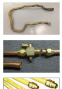
**Uncoated Brass Connectors**. These flexible, corrugated metal tubes are used to connect natural gas appliances to gas supply piping. Some older connectors made of uncoated brass have a serious flaw that could lead to a gas leak, fire or explosion.
