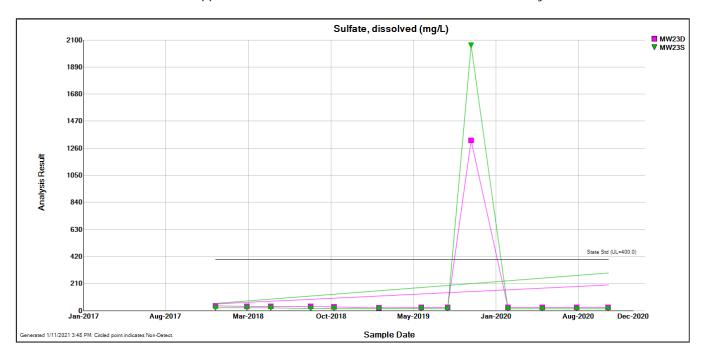
**Figure 1-12.** Sulfate concentrations since 2017 at compliance wells MW-23S and MW-23D. The Class I Groundwater Standard is not applicable within the GMZ and is shown for reference only.
