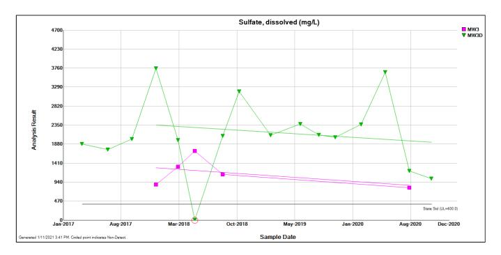
**Figure 1-9.** Sulfate concentrations since 2017 at compliance wells MW-3 and MW-3D. The Class I Groundwater Standard is not applicable within the GMZ and is shown for reference only. Circled results indicate non-detects.
