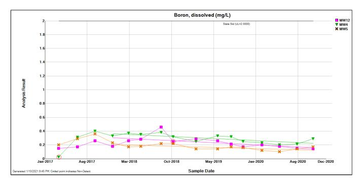
**Figure 1-5.** Boron concentrations since 2017 at compliance wells MW-4, MW-5 and MW-12. The Class I Groundwater Standard is not applicable within the GMZ and is shown for reference only. Circled results indicate non-detects.
