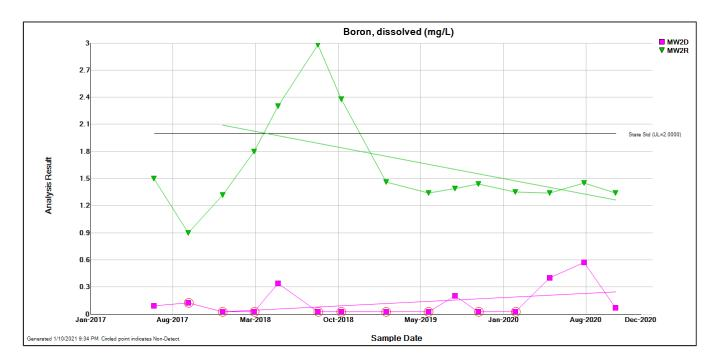
**Figure 1-3.** Boron concentrations since 2017 at compliance wells MW-2D and MW-2R. The Class I Groundwater Standard is not applicable within the GMZ and is shown for reference only. Circled results indicate non-detects.
