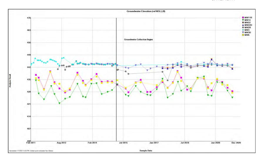
Figure 3-5. Groundwater elevations near groundwater collection trench
