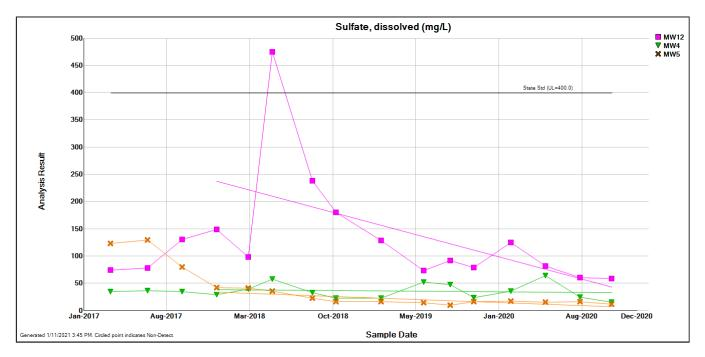
**Figure 1-10.** Sulfate concentrations since 2017 at compliance wells MW-4, MW-5 and MW-12. The Class I Groundwater Standard is not applicable within the GMZ and is shown for reference only.
