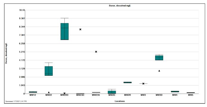
**Figure 3-6.** Box-whisker plot showing distribution of **boron** concentration by monitoring well for data collected in 2019 and 2020
