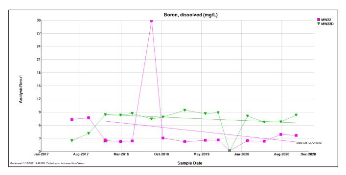
**Figure 1-6.** Boron concentrations since 2017 at compliance wells MW-22S and MW-22D. The Class I Groundwater Standard is not applicable within the GMZ and is shown for reference only. Circled results indicate non-detects.
