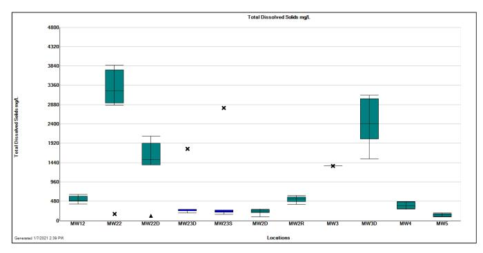
**Figure 3-12.** Box-whisker plot showing distribution of **total dissolved solids** concentration by monitoring well for data collected in 2019 and 2020.
