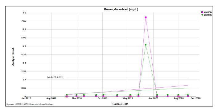
**Figure 1-7.** Boron concentrations since 2017 at compliance wells MW-23S and MW-23D. The Class I Groundwater Standard is not applicable within the GMZ and is shown for reference only. Circled results indicate non-detects.
