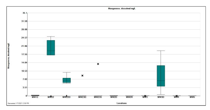
**Figure 3-10A.** Box-whisker plot showing distribution of **manganese** concentration by monitoring well for data collected in 2019 and 2020.
