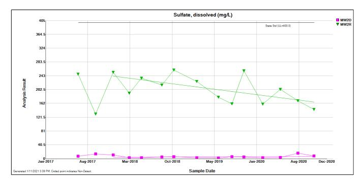
**Figure 1-8.** Sulfate concentrations since 2017 at compliance wells MW-2D and MW-2R. The Class I Groundwater Standard is not applicable within the GMZ and is shown for reference only.
