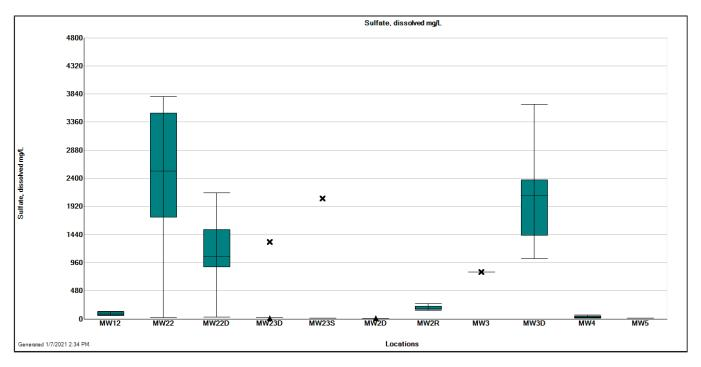
**Figure 3-8.** Box-whisker plot showing distribution of **sulfate** concentration by monitoring well for data collected in 2019 and 2020.
