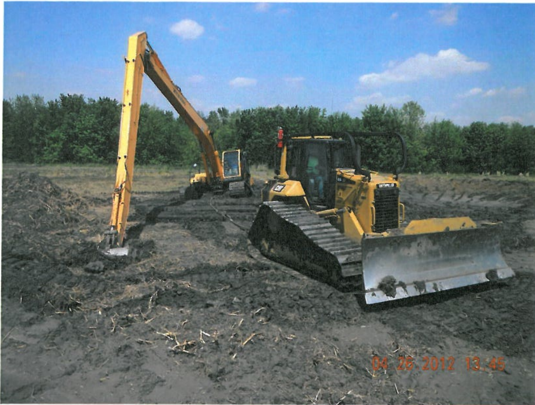
Photograph 9 ▲ - Long reach excavator stuck in wet ash, northeast corner of Ash Pond D facing northeast
