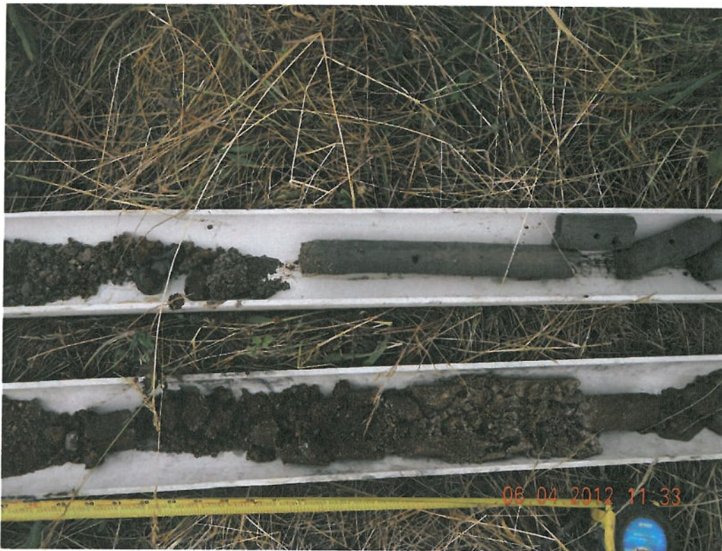
Photograph 4 ▲ - Soil samples from monitoring well MW-2R facing south
