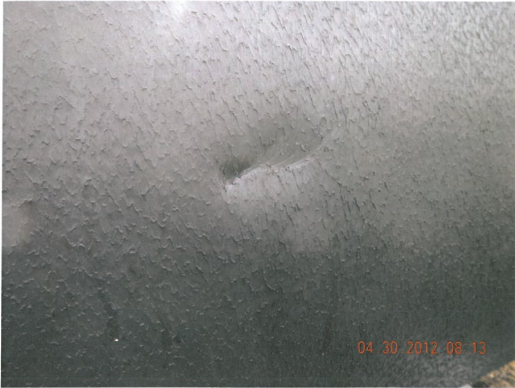
Photograph 3 ▲ - Example of dimple in roll facing east
