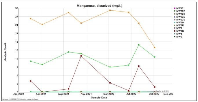
**Figure 3-11A. Manganese** concentrations during the reporting period (2021-2022) at all background and compliance wells. Note: Circled results indicate non-detects.
