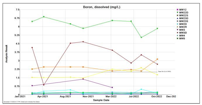
**Figure 3-7. Boron** concentrations during the reporting period (2021-2022) at all background and compliance wells. Note: Circled results indicate non-detects.
