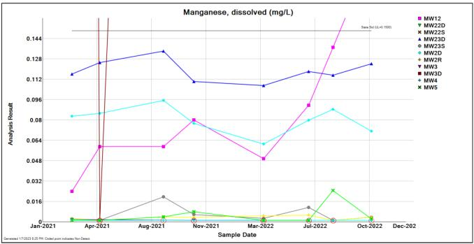
**Figure 3-11B. Manganese** concentrations during the reporting period (2021-2022) at all background and compliance wells. Zoomed in to show the Class I groundwater standard. Note: Circled results indicate non-detects.
