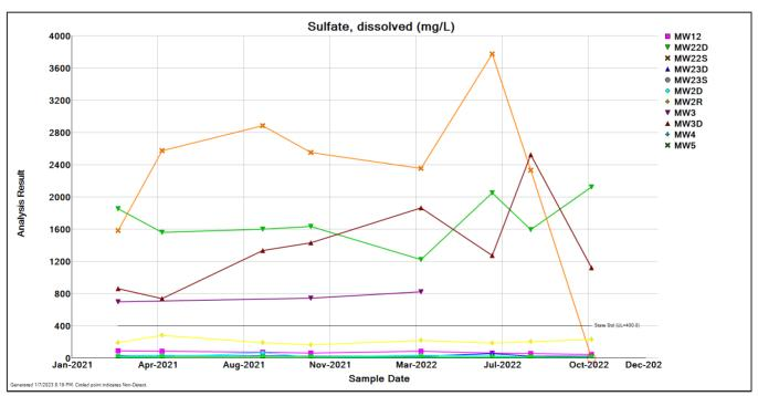
**Figure 3-9. Sulfate** concentrations during the reporting period (2021-2022) at all background and compliance wells.
