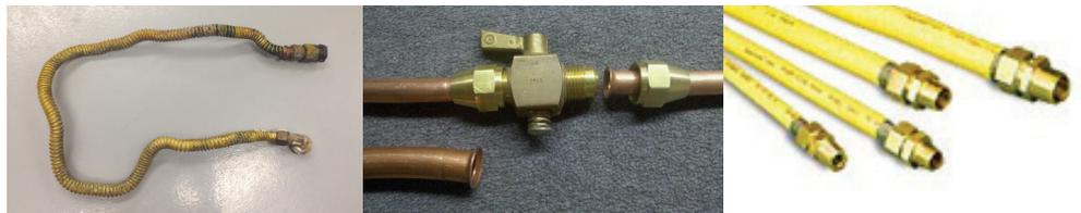
**Uncoated Brass Connectors:** These flexible, corrugated metal tubes are used to connect natural gas appliances to natural gas supply piping. Some older connectors made of uncoated brass have a serious flaw that could lead to a natural gas leak, fire or explosion.
