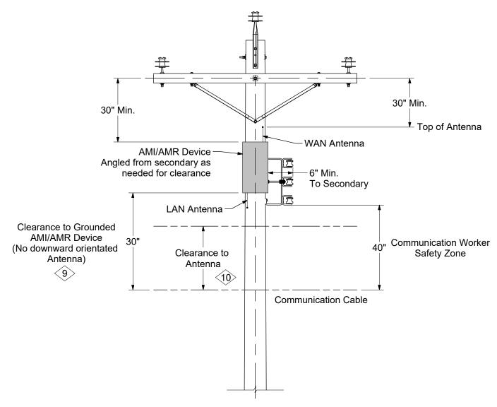
Antenna & AMI/AMR Device Clearances in 3 Phase Supply Space
