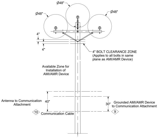
Antenna & AMI/AMR Device Supply Space Installation/Clearance Zone
