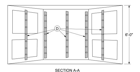
Side View of Cable Racks in Manhole
