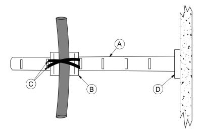
Cable / Splice Cross Tie Down Detail
