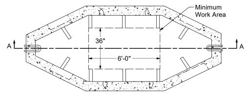
Cable Rack Spacing in Manhole
