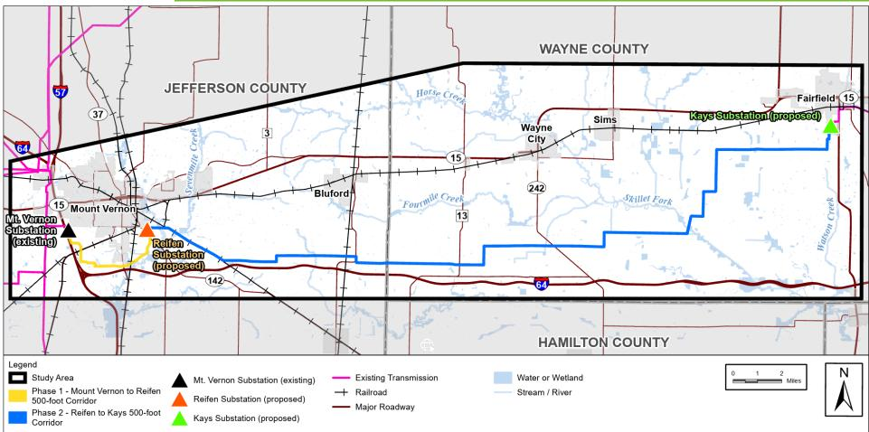
DISCLAIMER: This high-level map depicts the preferred route as a 500-foot wide corridor. The requested easement width for the transmission lines will be 100 feet for Phase 1 and 150 feet for Phase 2.
