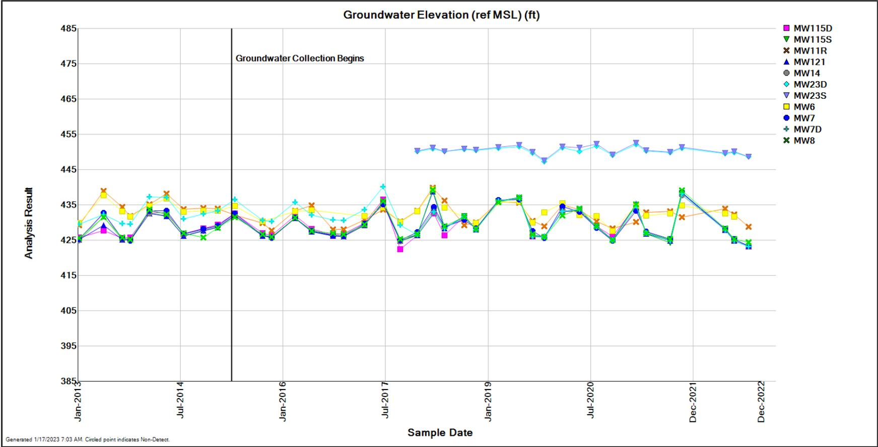
**Figure 3-5.** Groundwater elevations near groundwater collection trench.
