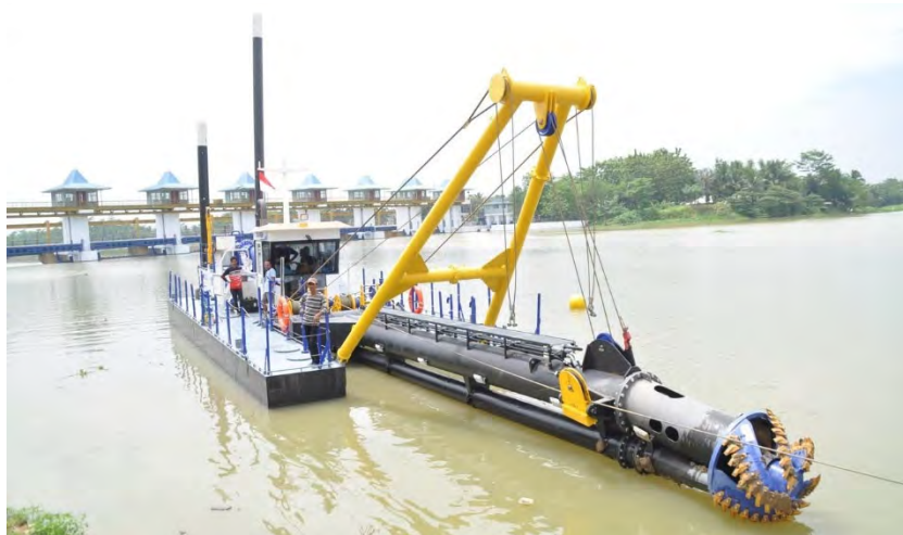
Figure 2 – Illustration of Cutter-Head Suction Dredge
