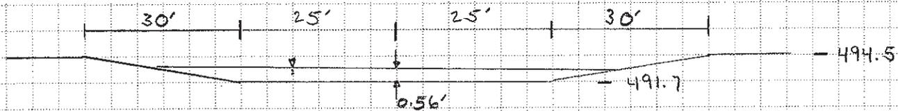
FOR MAX FLOW OF  $Q = 58.68$  cfs AND DEPTH  $D = 0.56$
