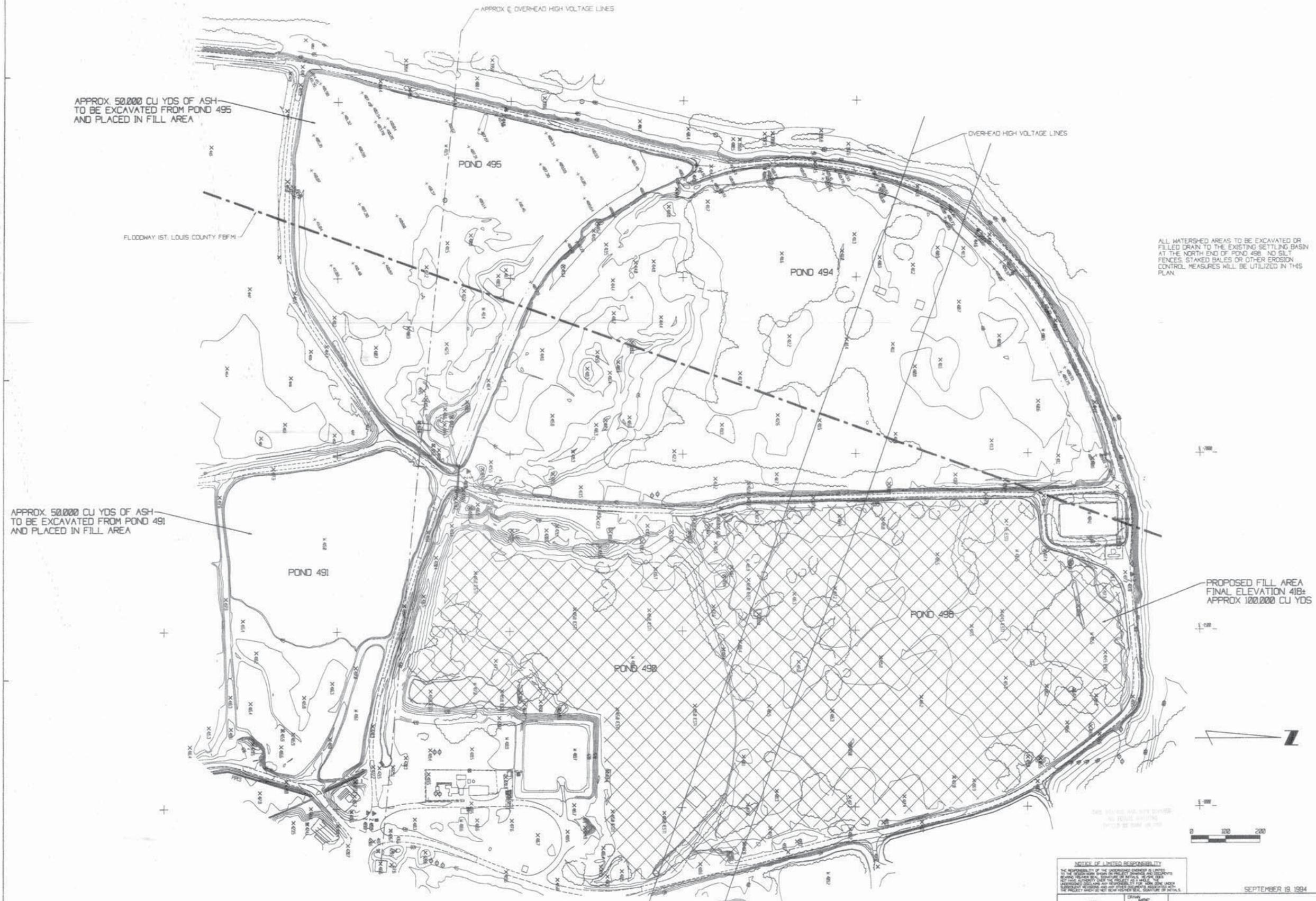
ALL WATERSHED AREAS TO BE EXCAVATED OR FILLED DRAIN TO THE EXISTING SETTLING BASIN AT THE NORTH END OF POND 496. NO SALT FENCES, STAKED BALES OR OTHER EROSION CONTROL MEASURES WILL BE UTILIZED IN THIS PLAN.
