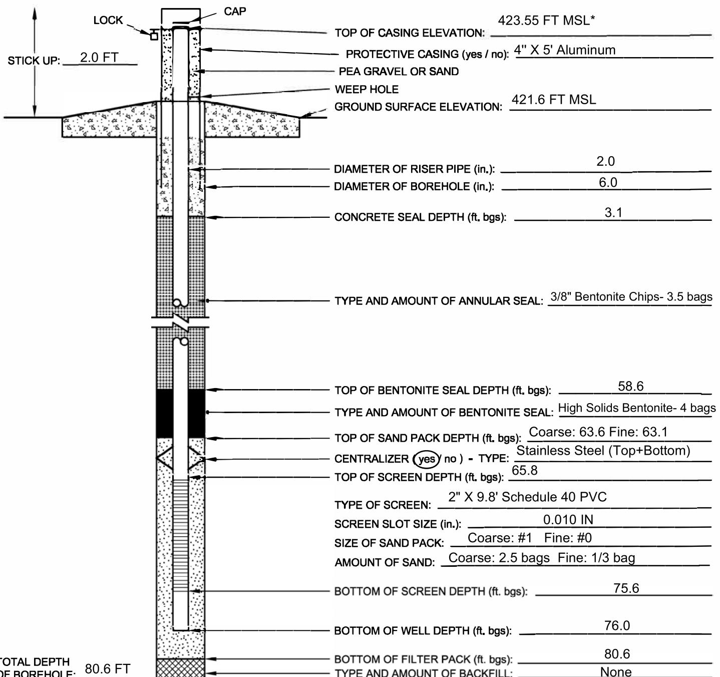
ADDITIONAL NOTES: FT BGS = Feet Below Ground Surface. FT MSL = Feet Above Mean Sea Level. FT BTOC = Feet Below Top of Casing.
