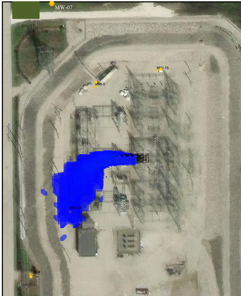
Figure 6a - Permanganate distribution following 365-day injection period with CW-04 on at 500 gpm and CW-05 off
