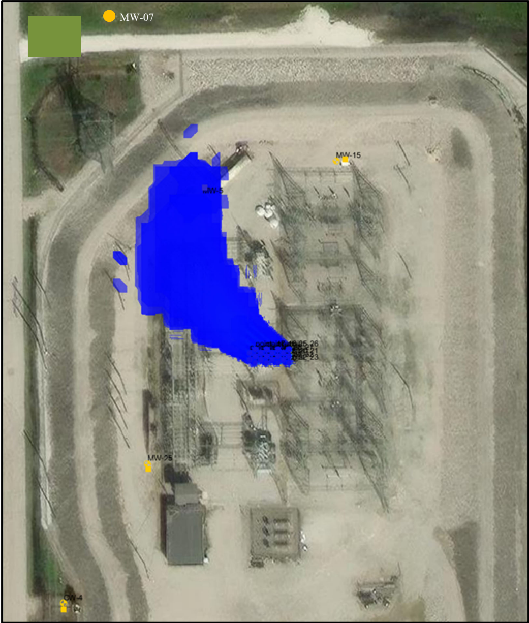
Figure 5a - Permanganate distribution following 365-day injection period with CW-04 & -05 operating at 500 gpm
