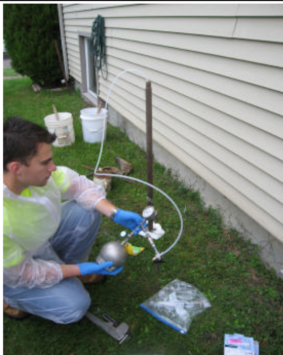
PHOTO 4: Obtain soil vapor sample in 1-Liter Summa Canister at VP505EWASH-2.
