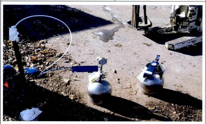
Photo 12: 504-N-12-Soil Vapor Sampling and Ambient Air Sampling
