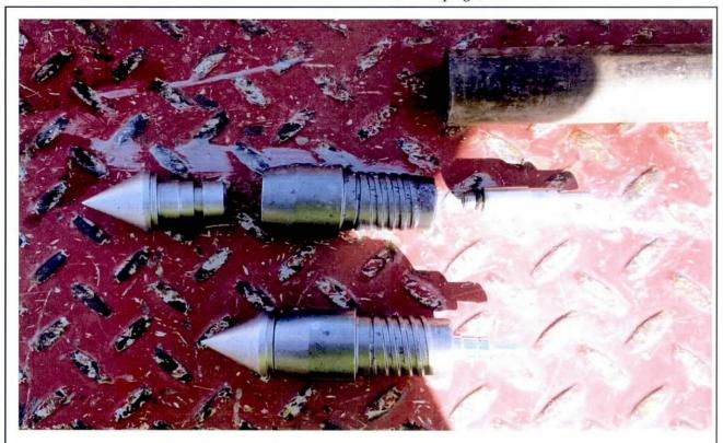
Photo 23: Post Run Tubing (PRT) Method Soil Vapor Sampling Assembly
