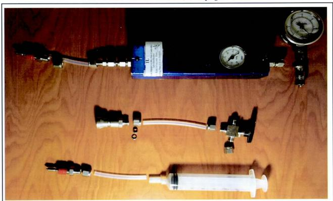
Photo 25: Soil Vapor Purging and Sampling Assembly
