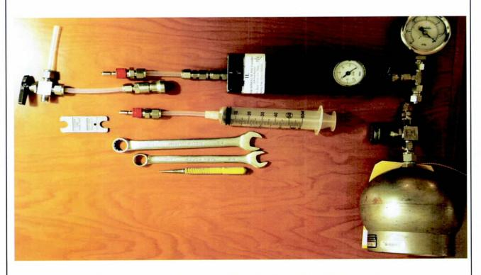
Photo 26: Soil Vapor Purging and Sampling Assembly with Summa Can
