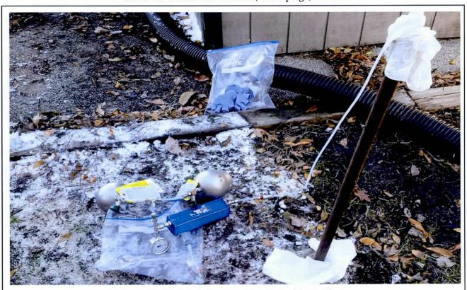
Photo 21: 508-N-9-Soil Vapor Sampling with Duplicate
