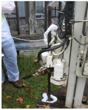
PHOTO 8: Another view of leak detector paper towels around rod on top of bentonite putty seal at VP412EHill-3 location.
