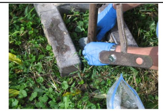
PHOTO 1: View of packing bentonite putty seal around probe.
