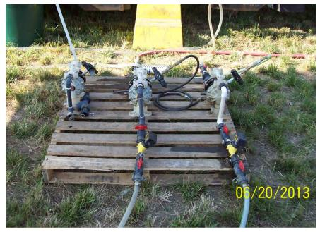
Above: Three air-operated double-diaphragm pumps, flow meters, and PVC reinforced tubing used for injections.
