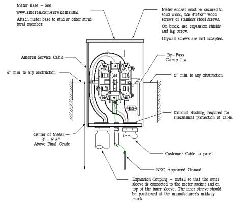
2. Metering equipment shall not be located on Company owned poles or on buildings adjacent to driveways, alleys, streets or other similar exposed places where it can be damaged by moving vehicles unless the equipment is protected by a substantial guard rail or posts. The customer shall consult the Company representative regarding providing adequate protected barrier
