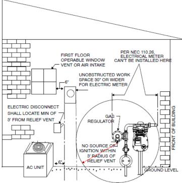
NOTE: METER EQUIPMENT'S LOCATION MUST SATISFY NEC 110.26, BOTH 3' VENT CLEARANCE TO GAS METER, AND 30" WORKING SPACE
