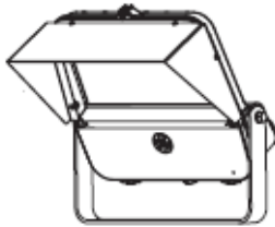
Figure 3-4. Light Shield ONLY needed based on request MUST SELECT THE CORRECT SHIELD FOR EACH MODEL OF LED LUMINAIRE SEE MODEL "(*)"
