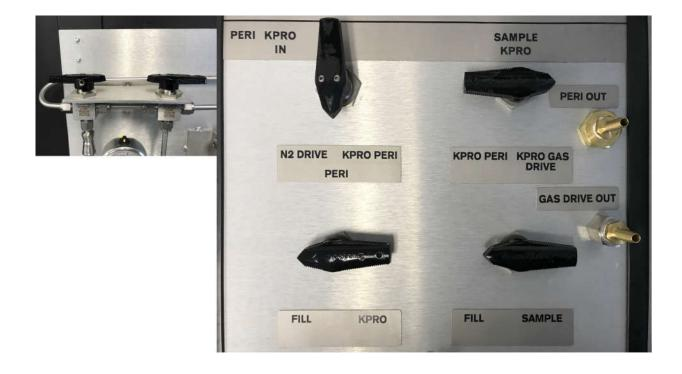
c. When a steady stream of water is flowing out of the Peri Out tubing on the APS box then the pump is full. Turn the two valves on the sample jig so that they are closed (facing the back of the box). Turn the bottom left valve 90 degrees to shut off the flow. Turn the top left valve to N2 Drive. Turn off the peristaltic pump. The pressure on the gauge will rise to where it is set on the regulator. Make sure the pressure is set to around 60-100 psi or the expected working pressure.
