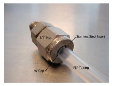
For the other end of the FEP, slide on another ¼" SwageLok<sup>®</sup> nut and ¼" nylon ferrule. Insert the end of the FEP into a ¼ "to <sup>1</sup>/<sub>8</sub>" SwageLok<sup>®</sup> reducer. Using a  $\frac{1}{2}$ " and  $\frac{9}{16}$ " wrench, tighten the nut as before. Be careful to keep the FEP seated tightly into the fitting while tightening. A completed tip can be seen in the following photo:
