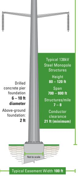
Note, this graphic is not to scale. The number of arms on a typical structure and the sizing of the structure may vary depending on the final route. Currently, there are existing Ameren transmission corridors in area that may provide an opportunity to co-locate lines along the same corridor or combine transmission lines onto one set of larger steel structures. This will be determined during the routing process.
