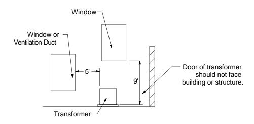
Typical Minimum Clearance Door and Window of Padmount Transformer
