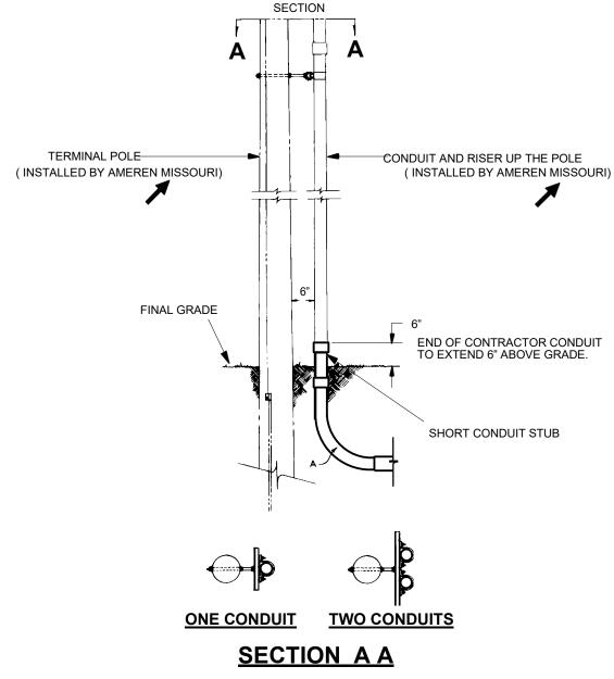
NOTE: AMEREN MISSOURI REP. WILL DESIGNATE THE QUADRANT OF THE POLE WHERE THE CONDUIT IS TO BE INSTALLED. MATERIAL INSTALLED BY CONTRACTOR FOR ONE RISER (DERIVED FROM CONSTRUCTION STANDARD 14 00 26 \*\* )
