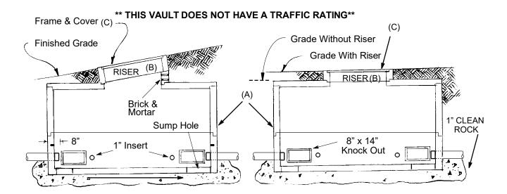
Grade adjustments shill be made using the riser and necessary brick and mortar to meet the existing slope. The vault floor shall always be installed level.
