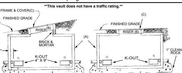
Grade adjustments shall be made using the riser and necessary brick and mortar to meet the existing slope. The vault floor shall always be installed level.
