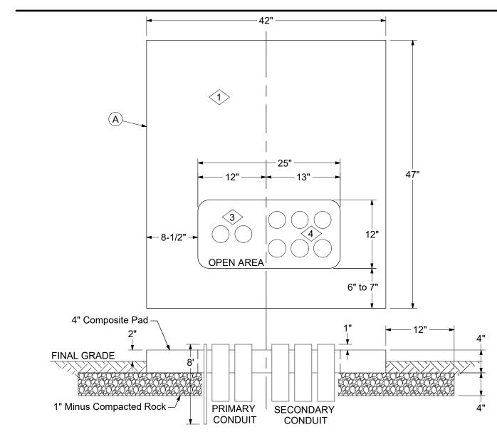
34 21 05 02 - Heavy Pad 25 kVA thru 250 kVA Single Phase Loop Feed
