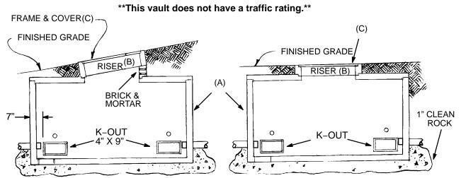
Grade adjustments shall be made using the riser and necessary brick and mortar to meet the existing slope. The vault floor shall always be installed level.
