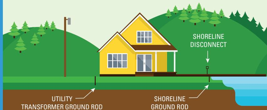
In order for your docks electrical system to function in a safe manner, the grounding system must be connected all the way back to the utility transformer. This is accomplished by testing the grounding system between the dock and the house panel box, not to the ground rod or shoreline disconnect near the seawall. This test should show that there is less than 1 ohms resistance on the grounding system.
